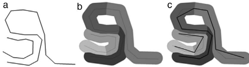
Fig. 3. Polyline simplification procedure. (a) Original polylines. (b) \epsilon -Voronoi diagrams of monotone sub-polylines. (c) Ultimate simplified results (bold black lines).
