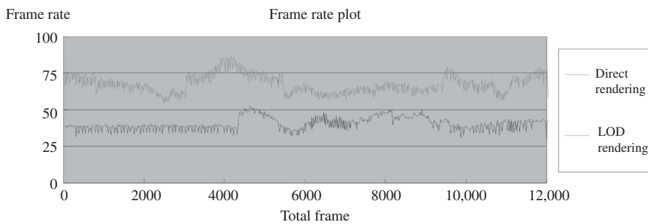
Figure 12. Comparison of frame rates between rendering the origin building models and LOD models.
